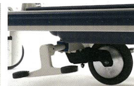
Training Wheels for Going Straight Training wheels for going straight are installed in the middle of the car so that, it can be easily operated to go straight and also circumvolve on the spot treating the training wheels as its axis
