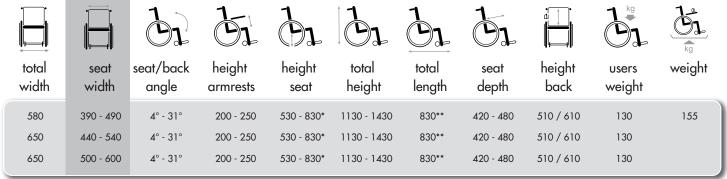
Sizes in mm, weight in kg - \* Without seat cushion - \*\* Without foot rests - Deviations in sizes and weight (15 mm, 1,5 kg, 1,5°) are possible.
